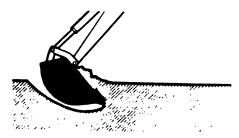
When digging in hard-packed soil, bucket penetration can be increased by applying down pressure with the boom while crowding in and curling the bucket. If the crowd action "stalls" it may be necessary to apply lift occasionally during the digging cycle to correct the bucket depth.
